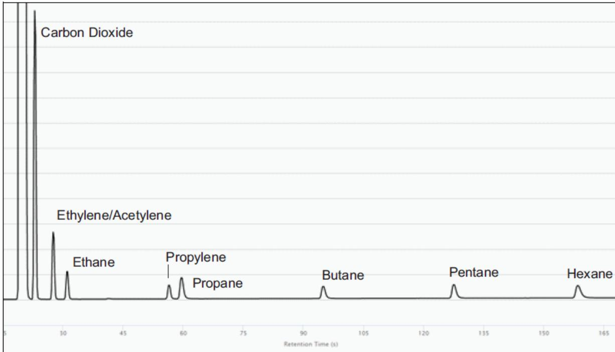
Column Temperature: 60°C (hold 20 seconds) → 200°C (hold 10 seconds); Ramp Rate: 1.0°C/s;
