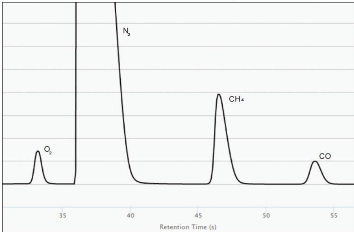
Column Temperature: 110°C (hold 30 seconds) → 200°C (hold 20 seconds); Ramp Rate: 1.5°C/s;
