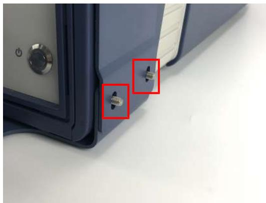
8 Place the wing nuts on the bottom bracket threads and hand-tighten. Ensure that the top bracket is pressed downward and is tightly secured to Micro GC Fusion.
