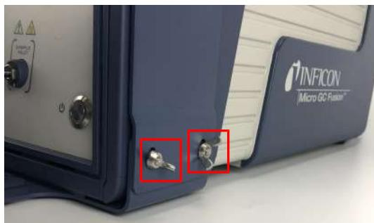
9 Using a 3 mm hex driver, slightly thread the M4 screws into the holes on the bottom bracket, near the chassis of Micro GC Fusion.
