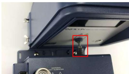
12 Loosely thread the front screws into the slide plate using a 3.0 mm hex driver.
