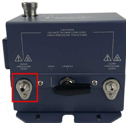
17 Attach a 1/16 in. vent line to the LOW PRESSURE VENT. Tighten it with a 5/16 in. open-ended wrench.
