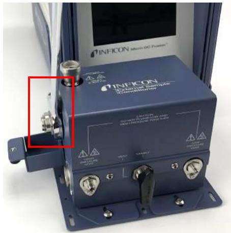
**12** Cover the bonnet nut by reattaching the cover door using the thumb screw on the side of the device.
