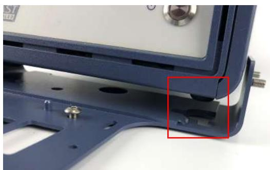
6 Slide the top bracket over Micro GC Fusion and the threads from the bottom bracket.
