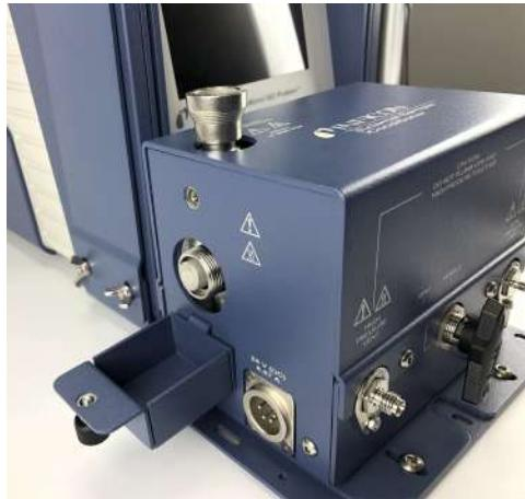
The filter assembly nut is tightened 1/8 turn past finger-tight for high pressure applications.
