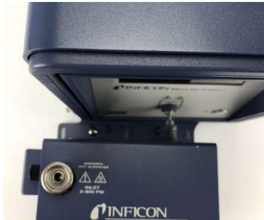
11 Gently push the device toward the instrument until the transfer line reaches the front inlet of Micro GC Fusion.
