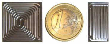
Figure 1 - Pre-concentrator and MEMS chromatographic gas column
