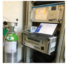
Figure 2 - Installation of the PyxisGC BTEX in the cabin
